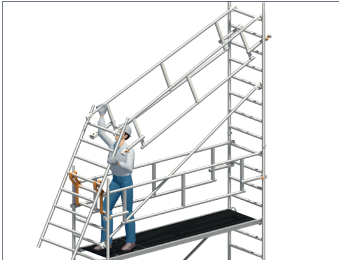
1. Attach the first ladder frame. Attach the Uni assembly hooks and position the second ladder frame in order to fit the double guardrail on both sides.
