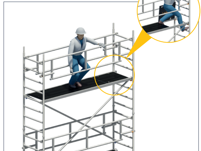
4. Access to the already secured level and final snapping into place of the double guardrail (lower snap-on claws) into the ladder frame.
