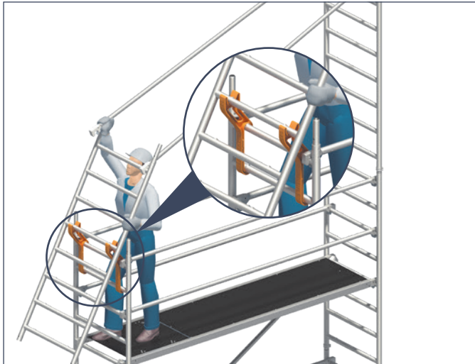
1. Attach the first ladder frame. Attach the Uni assembly hooks and position the second ladder frame in order to fit the guardrails.
