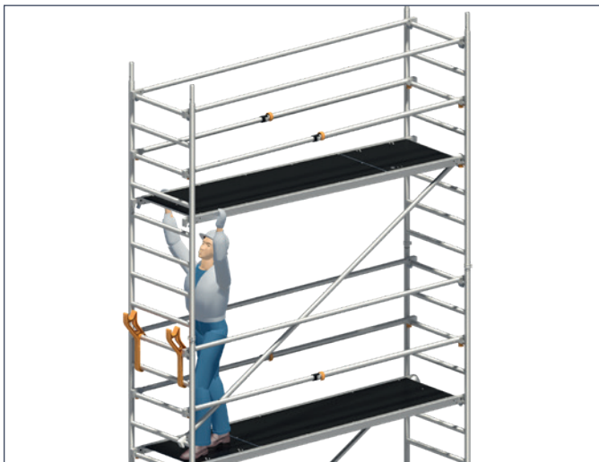
3. Insert diagonal braces and access deck.
